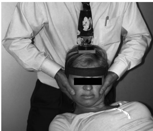
Figure 1 Flexion-rotation test measurement position and modified cervical range of motion measurement device.
